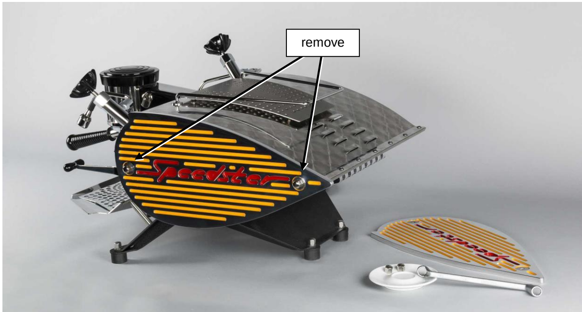
Figure M 1. To remove side panel loosen the 2 nuts with a 13 mm spanner.
