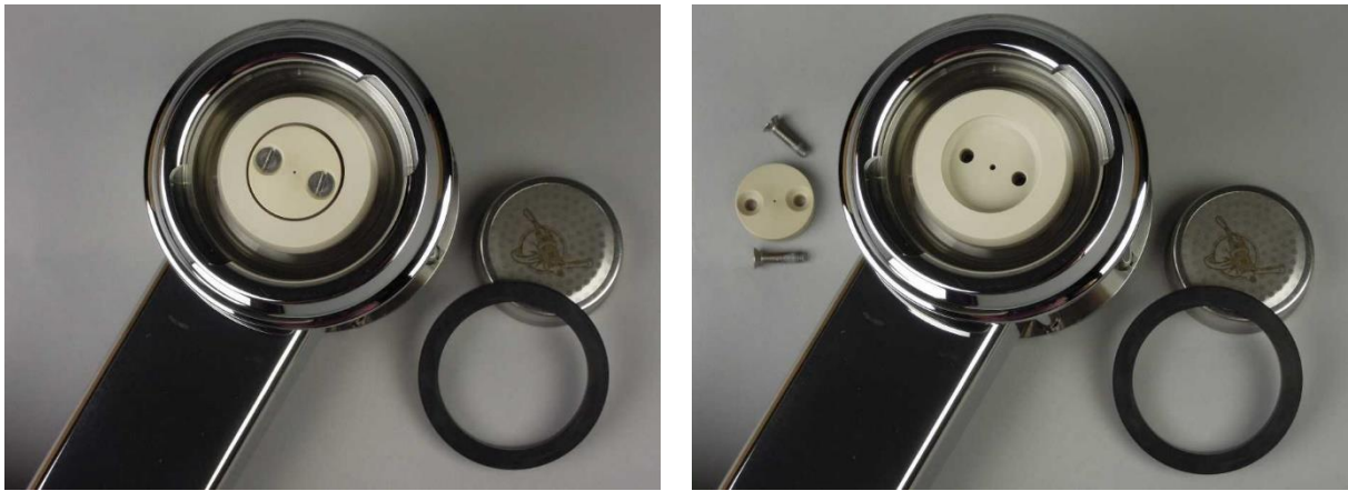
Figure 18. Shows dispersion plate mounted with 2 screws (left) and dispersion plate removed from group (right). Photos taken from bare coffee-boiler laying on its back.
