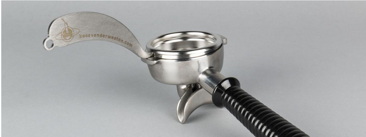
Figure 16. Pry filter basket from filter holder with the group screen extractor.
