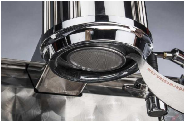
Figure 17. Left: Gently pry left and right with group screen extractor to remove group screen and group seal.
