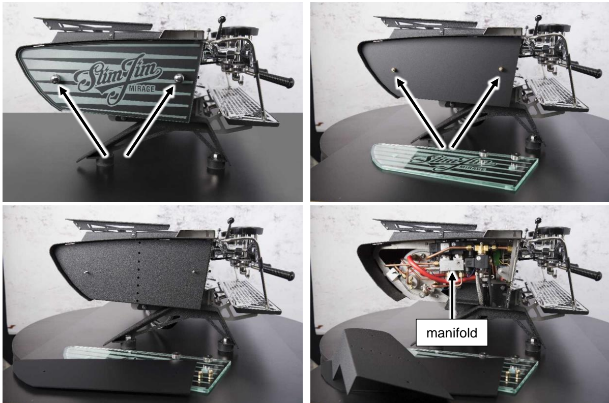
Figure 13. Undo the nuts and remove the left-hand side panel (when glass side panels are mounted you have to remove the underlying support nuts as well to be able to remove the inner panel).
