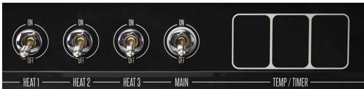
Figure 7. Showing the three HEAT switches, the MAIN switch and a blank TEMP/TIMER (3-digit) display.
