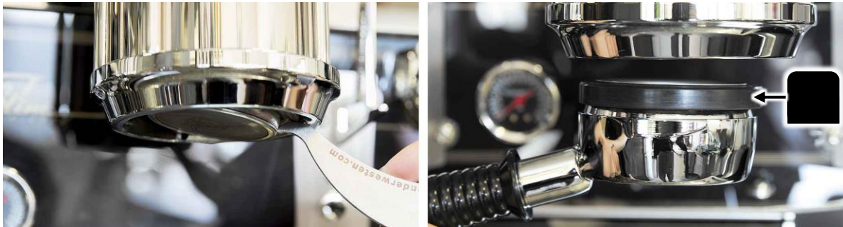
Figure 22 a (left). Pry left and right with screen extractor to remove group screen and group seal.
