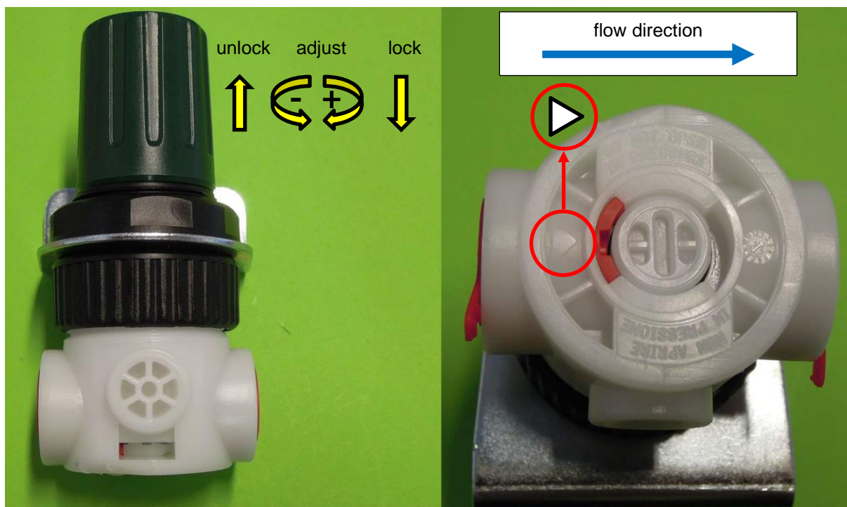
Figure 19. How to adjust the Vesta pressure reducer setting; procedure for the AIGNEP version is similar. Pull the knob out and then twist to the correct setting. When done, push the knob back in. Note that the machine will not lose pressure due to one-way valves in the system. Set the outgoing pressure during an actual brew (not with a blind filter).
