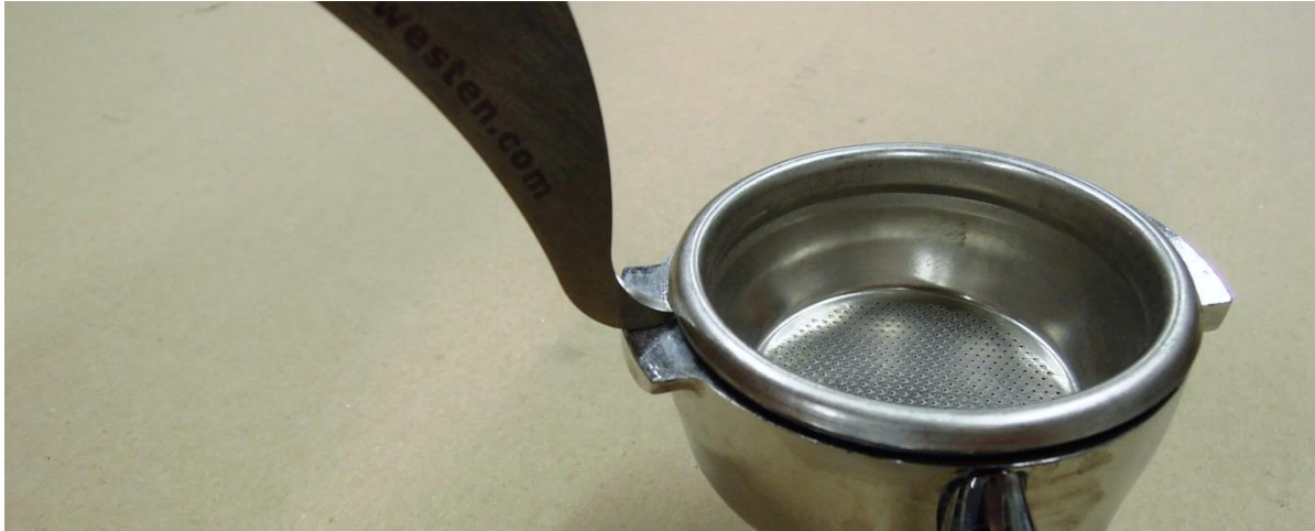
Figure 21. Pry filter basket from filter holder with the group screen extractor.
