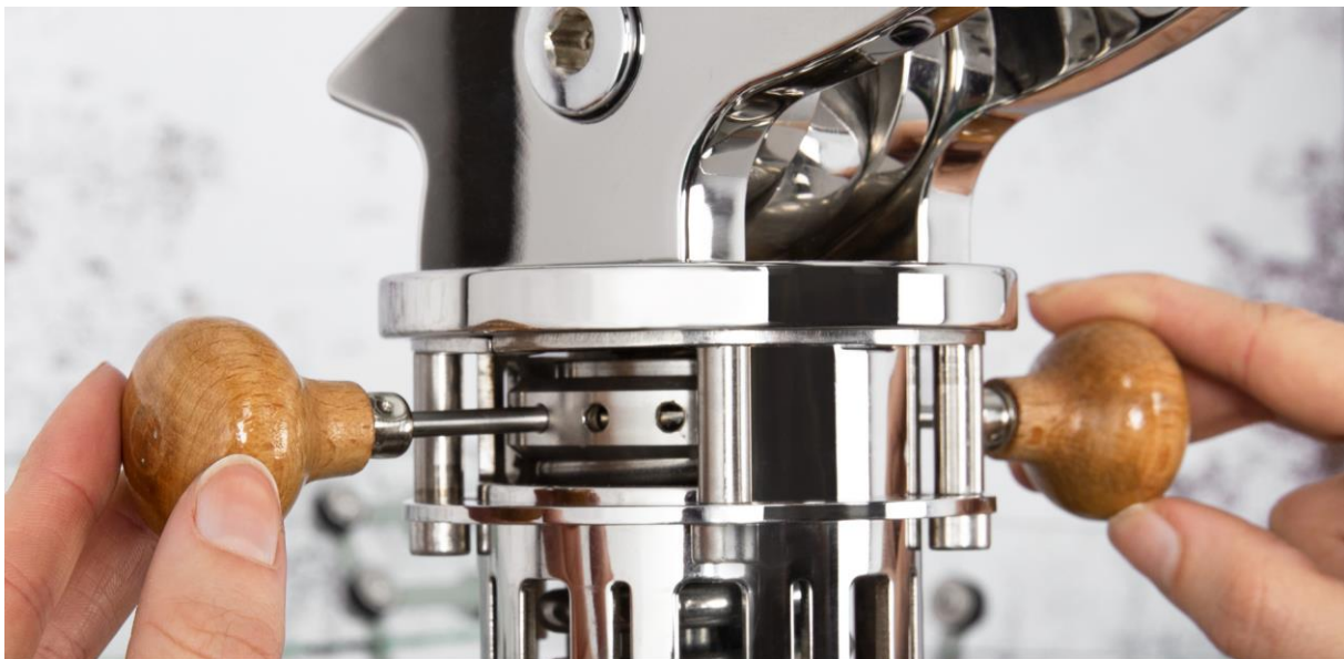
Figure 10. The spring-length adjuster disk. Insert a tool in one slot on each side of the group, use these to twist the disk.
