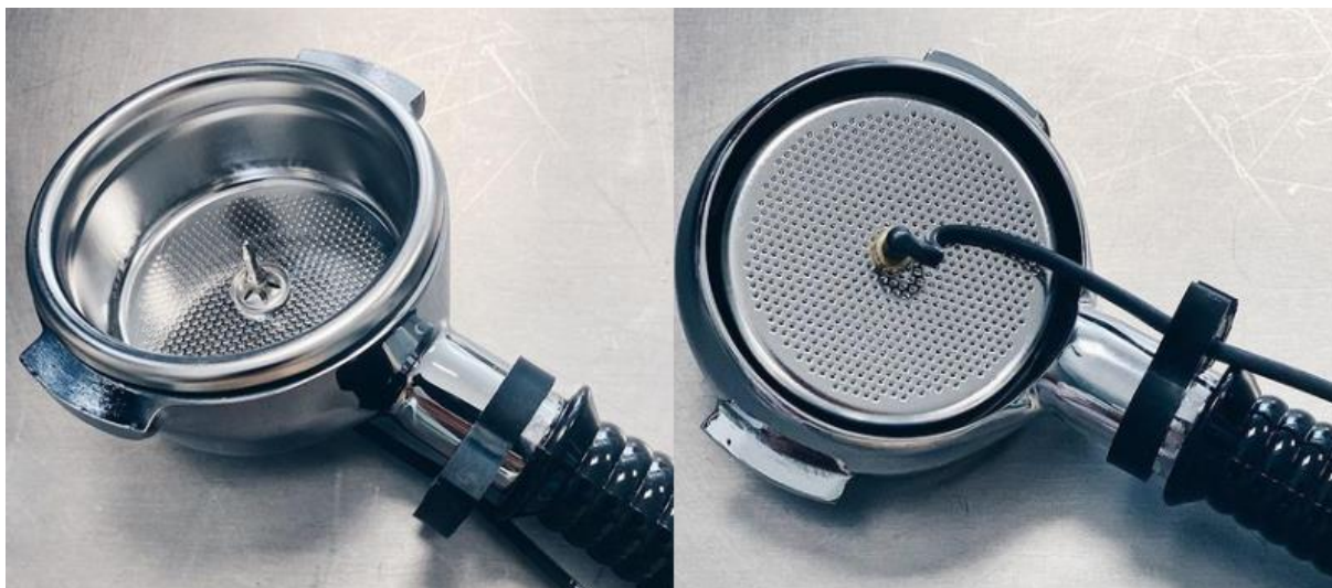
Figure 17. Temperature sensor in filter basket (K03344-00 mounted in bottomless portafilter).
