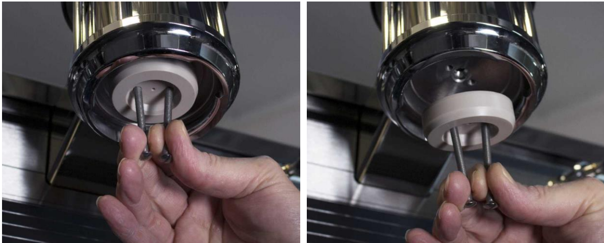
Figure 27. How to remove the dispersion base. Use 2 bolts M5x60 or similar to get grip onto the dispersion base.
