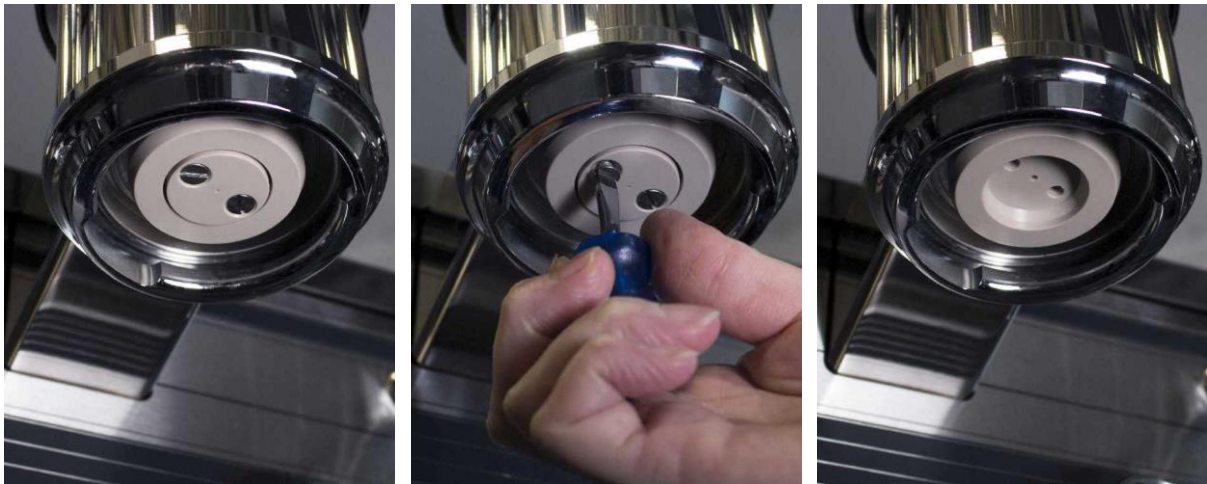
Figure 26. Dispersion set mounted in group head. Remove the 2 screws. The dispersion plate will fall out. The dispersion base remains in the group.
