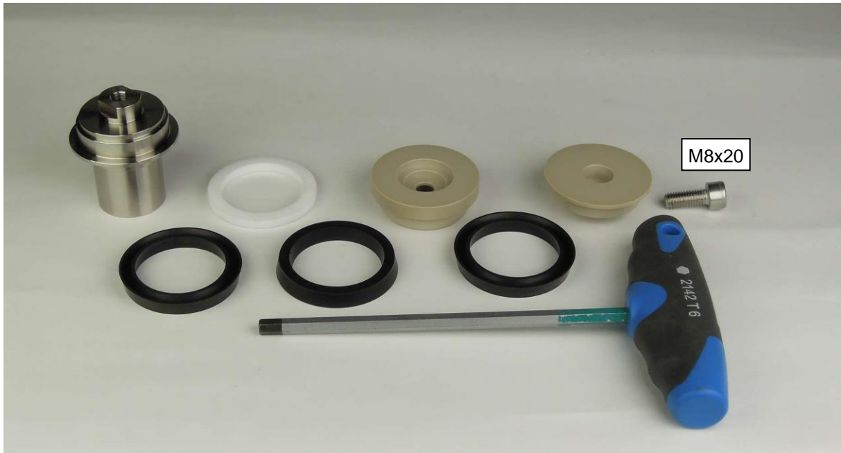
Figure 24. The piston taken apart. Normally the group head, piston-rod, spring and piston remain assembled.
