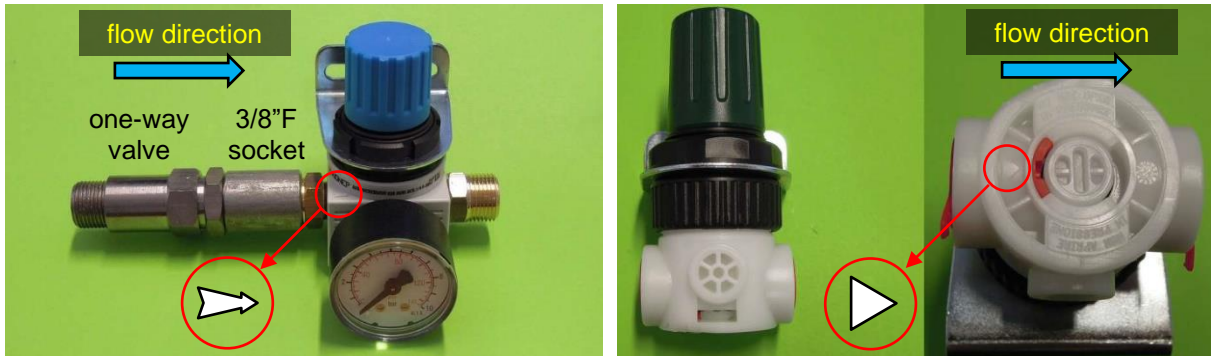
Figure 14. The AIGNEP (left, with one-way valve and socket) and Vesta (right) pressure reducer.
