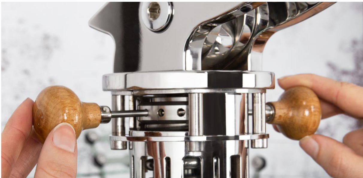
Figure 25. The spring-length adjuster disk. Insert a tool in one slot on each side of the group, use these to twist the disk.
