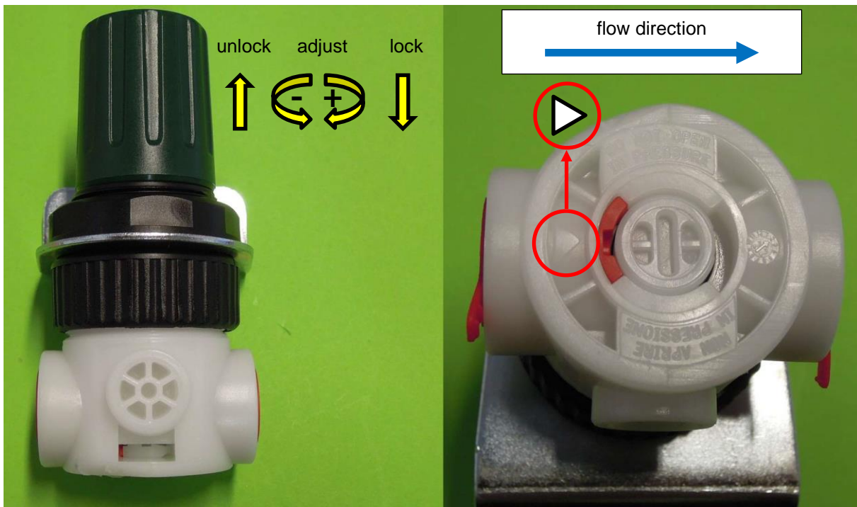
Figure 20. How to adjust the Vesta pressure reducer setting; procedure for the AIGNEP version is similar. Pull the knob out and then twist to the correct setting. When done, push the knob back in. Note that the machine will not lose pressure due to one-way valves in the system. Set the outgoing pressure during an actual brew (not with a blind filter).
