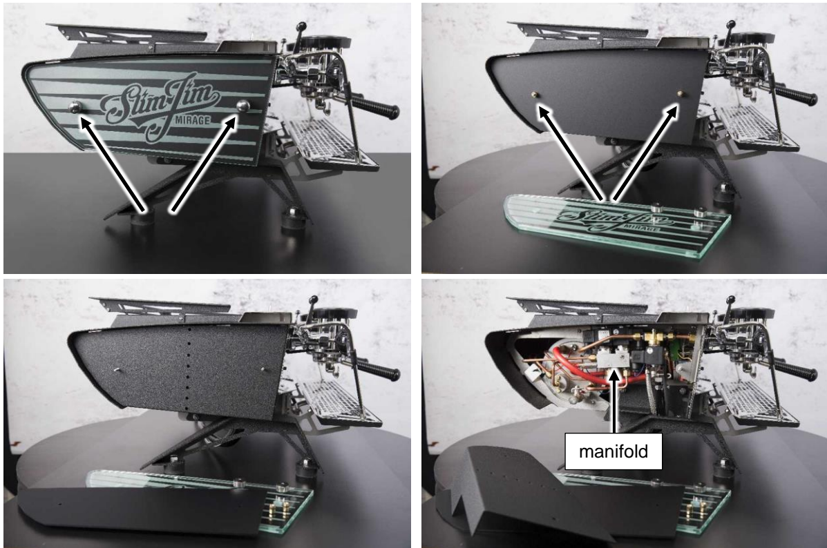
Figure 23. Undo the nuts and remove the left-hand side panel (when glass side panels are mounted you have to remove the underlying support nuts as well to be able to remove the inner panel).
