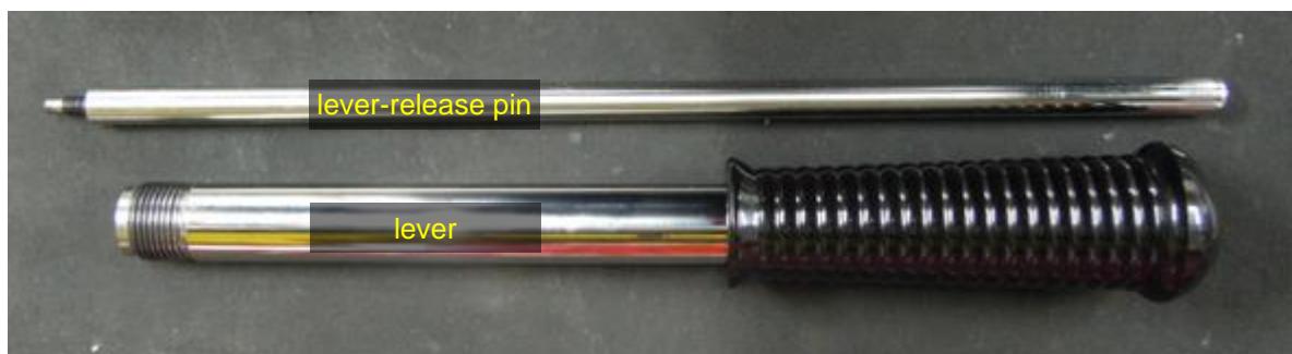
Figure 11. Showing the lever release pin (top) and lever (bottom).
