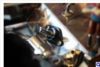
Preinfusion Piston Piston is fully engaged (sticking out of the machine) showing full preinfusion.
