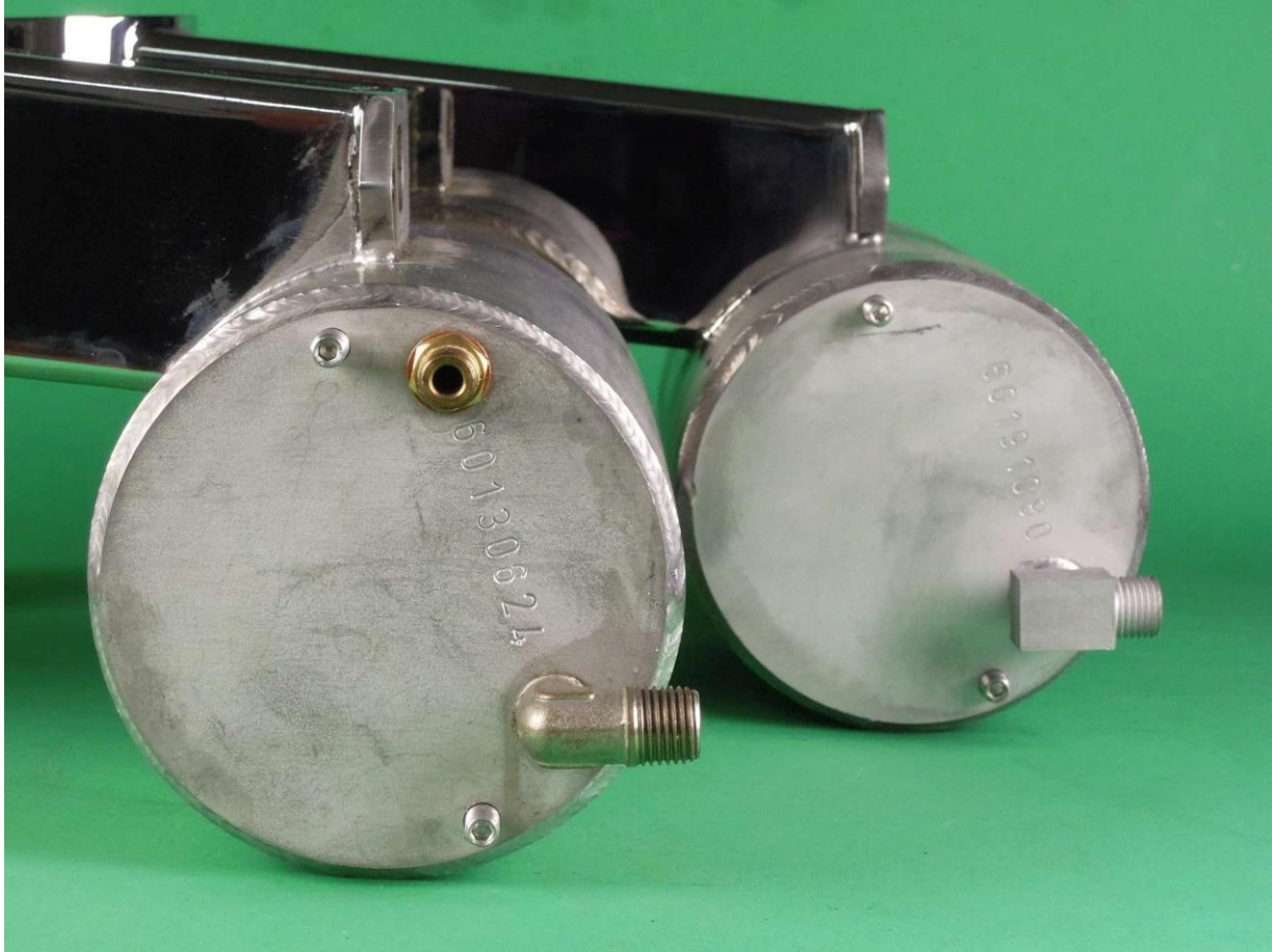
Left: coffee boiler (# 190-629) with 1/8M-1/8M brass fitting for PPIC and injection line (not visible) in 1/8M-1/8M nickel-plated brass knee-fitting. Used until October 2016. Right: 2017 version coffee boiler (# 630-...) with welded-on stainless "knee-fitting with injection line".
